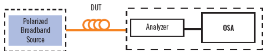
Fixed Analyzer method Principle
