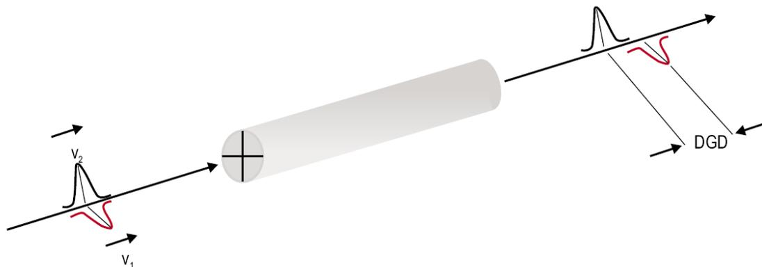
Figure 2: Differential group delay in HiBi fiber
